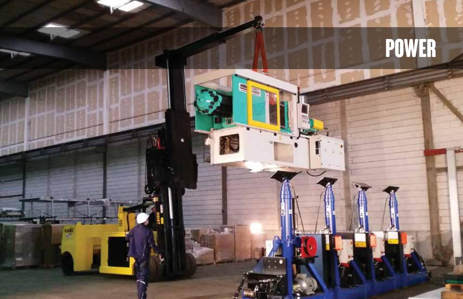
The FR Series is powered by a high-performance dual-fuel GM LPG engine and two-speed hydrostatic drive with variable RPM control. The “on-demand” hydrostatic drive pump offers not only power, but also increased productivity and fuel efficiency.
